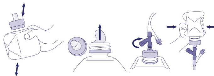
Figure 2. New cap-based bolus feeding system securely fixed onto collapsible semi-rigid bottles directly connectable to ENFit feeding tube
